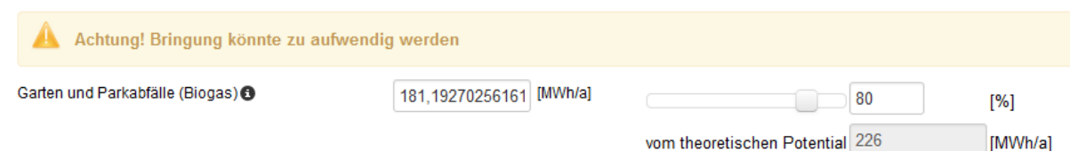
Figure 5: Excerpt of the benchmarking of biomass. The user intended to use more waste from parks as it is possible to collect with usual technologies. So RESYS warns the user.
